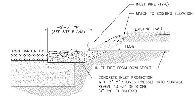
3 INLET PROTECTION CROSS-SECTION
